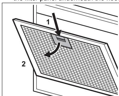
2. Slightly tilt the front of the filter downwards (2), then pull. Repeat the first two steps for all filters.
