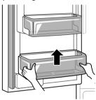
**2** To assemble the baskets, slide it in above the desired support and push down until it snaps into place.
