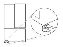
2 Open both doors and check to make sure that they close easily. If the doors do not close easily, tilt the appliance slightly more to the rear by turning both levelling legs to the left. It may take several more turns, and be sure to turn both levelling legs the same amount.
