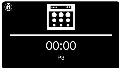
When the door is unlocked and can be opened, the
